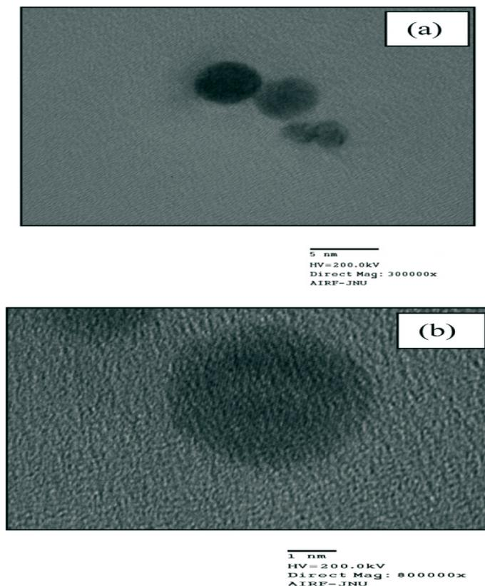
**Figure 2:** TEM images of silver nanoparticles at (a) 5 nm scale and (b) 1 nm scale [46].
