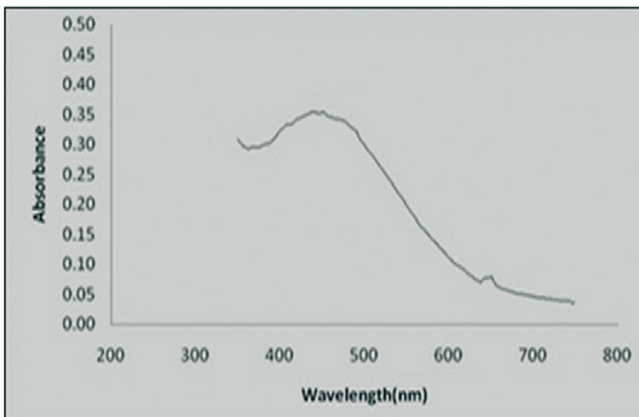
**Figure: 1** UV-Visible absorption spectra of colloidal solution synthesized AgNPs as a function of the wavelength in the range of 300–800 nm[46].
