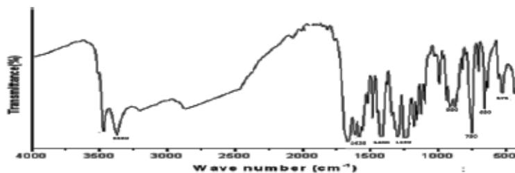
IR: The absorption band at 1638cm<sup>-1</sup>, is assigned to ν(C=N) stretching vibration, a feature found in Schiff bases. IR absorption at 3350 cm<sup>-1</sup>, characteristic of the carboxylic acid group. IR absorption spectrum of the Schiff base ligand shows a band at 1400 cm<sup>-1</sup>, characteristic of the ν(C=O) group. Mass: m/z 255
