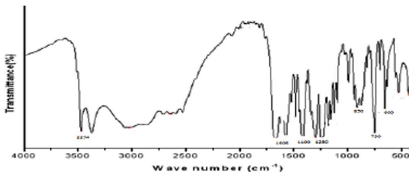
IR: Band at 1606 cm<sup>-1</sup>, which is assigned to  $\nu(\text{C}=\text{N})$  stretching vibration, a feature found in Schiff bases. IR absorption 1400 cm<sup>-1</sup>, characteristic of the  $\nu(\text{C}=\text{O})$  group. IR absorption at 3378 cm<sup>-1</sup>, characteristic of the carboxylic acid group. Mass:  $m/z=271$
