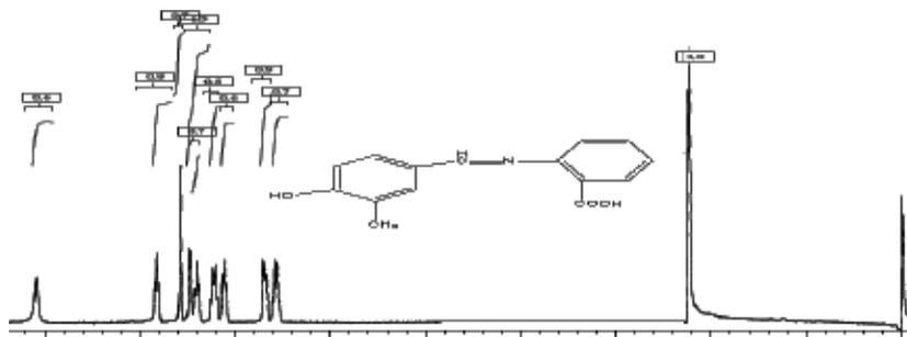
NMR: In the <sup>1</sup>H NMR spectra, the aromatic protons (7H) are observed in the range of 6.5 to 7.9 ppm. The azomethine proton (1H, N=CH) is observed at 7.4 ppm, and the carboxylic proton appears as a broad signal at 9 ppm. Methyl proton at 2.2ppm.
