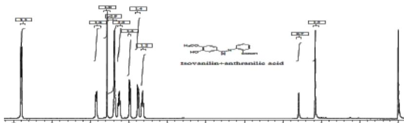
NMR: The aromatic protons (7H) are observed in the range of 6.56 to 7.8 ppm. The azomethine proton (1H, N=CH) is observed at 7.4 ppm, and the carboxylic proton appears as a broad signal at 9.8 ppm. Alcohol proton appears as a broad signal at 2.8 ppm. Methoxy proton appears as a broad signal at 2.2 ppm.
