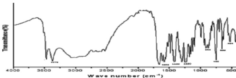
IR: The IR spectral data of the Schiff base showed a band at  $1606\text{ cm}^{-1}$ , which is assigned to  $\nu(\text{C}=\text{N})$  stretching vibration, a feature found in Schiff bases. IR absorption band at  $1400\text{ cm}^{-1}$ , characteristic of the  $\nu(\text{C}=\text{O})$  group. IR absorption band at  $3378\text{ cm}^{-1}$ , characteristic of the carboxylic acid group. Mass  $m/z=226$ .
