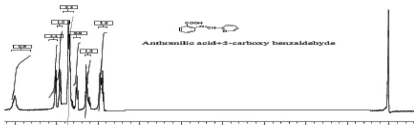
NMR: The aromatic protons (8H) are observed in the range of 6.9 to 7.3 ppm. The azomethine proton (1H,  $\text{N}=\text{CH}$ ) is observed at 7.4 ppm, and the carboxylic proton appears as a broad signal at 9 ppm.
