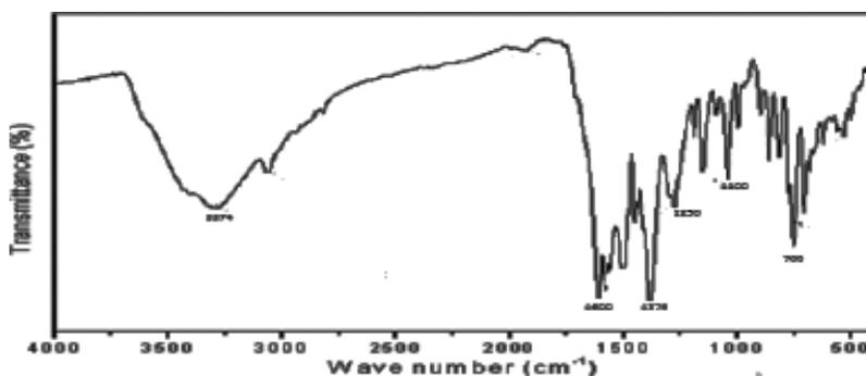
IR: Band at  $1600\text{cm}^{-1}$ , which is assigned to  $\nu(\text{C}=\text{N})$  stretching vibration, a feature found in Schiff bases. Band at  $1379\text{ cm}^{-1}$ , characteristic of the  $\nu(\text{C}=\text{O})$  group. Carboxylic acid group at  $3374\text{ cm}^{-1}$ . Mass:  $m/z=269$
